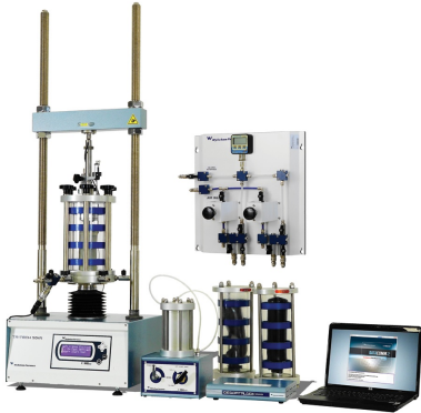
Standard triaxial system external/expandable data acquisition and air/water interface pressure system
